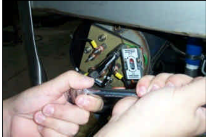
Removing the thermostat bracket/heater nuts.
